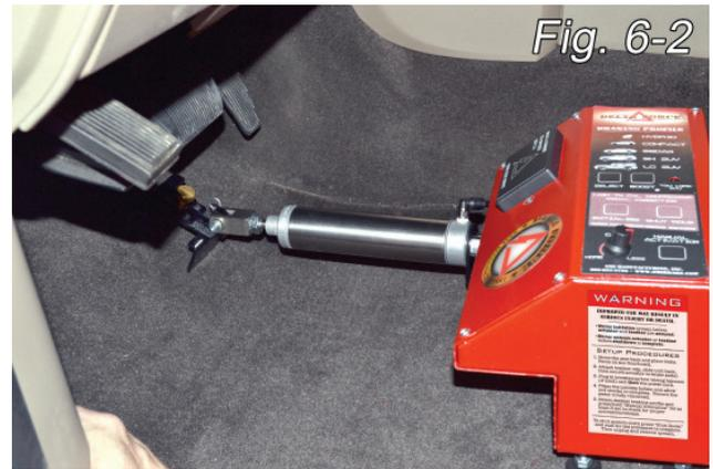
2. Rotate the actuator 90\* and allow the tether bracket to rotate downward (Fig. 6-2).
