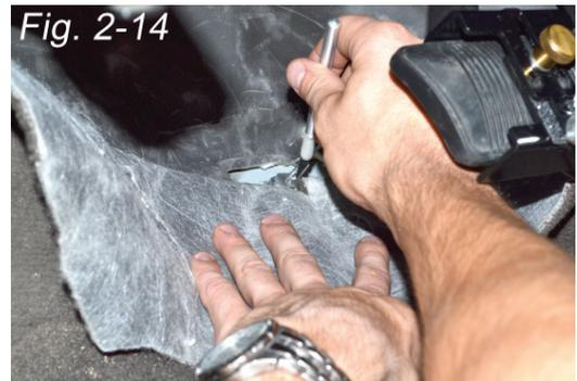
4. Trim or tuck in excess cable and fold carpet back and reattach carabiner to the actuator and secure pedal clamp to brake pedal.
