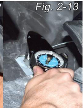
3. Slowly roll carpet back until the bend is resting over the cable. Pinch carpet and make a small slit from the back side of the carpet. Fold the carpet back and confirm that the slit is resting over the anchor. Cut a 1" slit downward. Pull the carpet back down and pass the carabiner through the slit.
