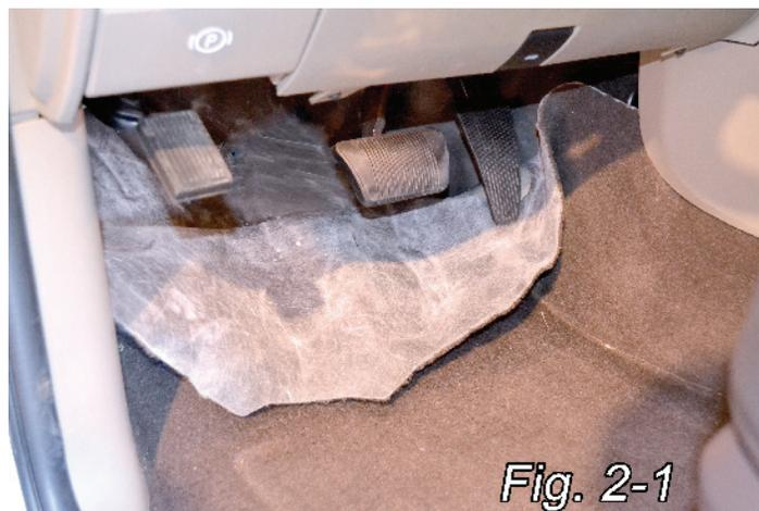
1. Pull back the carpet under the dash below the brake pedal to reveal the firewall insulation (Fig 2-1)
