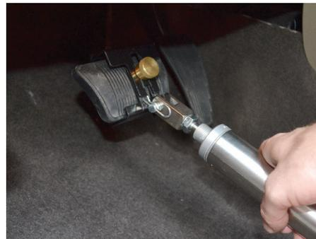
5. Check cable tension. If cable does not move 1/4" in either direction freely the cable needs to be loosened. If it moves more than 1" in either direct it needs to be tightened. (Cable adjustment shouldn't need to be changed after initial setup.)
