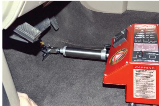
1. Place Delta Force on the floorboard in front of the driver's seat.
