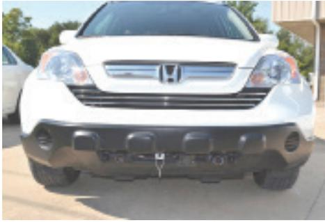
1. Mount the breakaway switch to the front of the towed vehicle as close to the center of the towed vehicle as possible using the provided hardware. In many cases it can be mounted to the front fascia in a manner that allows it to turn 90\* when not in tow.
