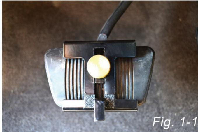
1. Loosen knob so the top and bottom brackets move freely and place Set-It-Once Pedal Clamp™ on brake pedal (Fig. 1-1).
